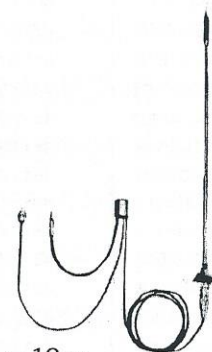
CB/VHF Cowl-Mount For mobile use. Chrome telescopic whip (50" extended, 28" collapsed), mounted on swivel base. Weatherproof loading coil. 22' RG-58/U cable. Terminates with PL-259 and pintype plug connectors. Catalog Number 21-930
